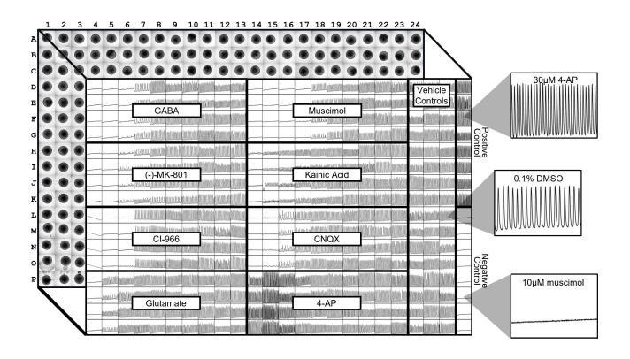
384-wells of functional activity can be captured simultaneously using high-throughput kinetic plate readers such as FLIPR. Shown above are the dose-dependent changes in waveform activity in response to 8 neuromodulators including positive control K+ blocker, 4-AP, and GABA analog, muscimol. The waveforms demonstrate remarkable reproducibility between replicates, enabling the use of as few as 4 organoids per condition.
